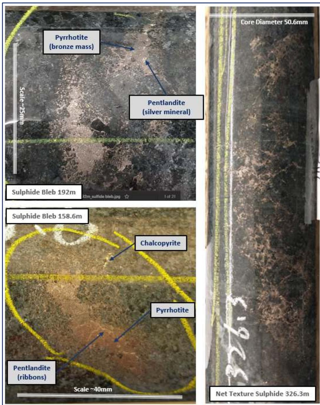
**Figure 2** – FLC2022-045 core photos of typical sulphide mineralisation – Pentlandite (Ni sulphide), Chalcopyrite (Cu sulphide) and Pyrrhotite (Fe sulphide) within Olivine Pyroxenite host rock
