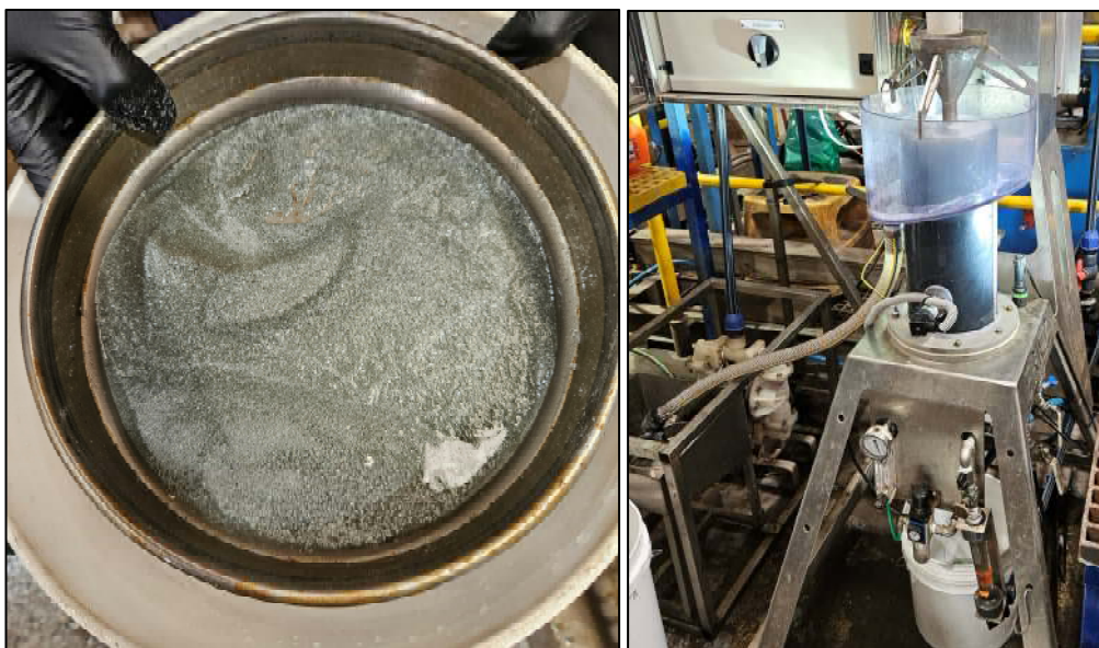
Figure 3 – (Left) Concentrate produced from the HydroFloat testwork. (Right) Eriez HydroFloat test unit.
