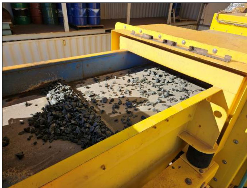
Figure 2 – Steinert Ore Sorter Vibrating Feeder.
