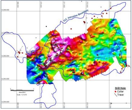
**Figure 7** – IP Chargeability Image – 2016-2017 2D ground IP geophysical surveys. Hot colours depict strong IP chargeability, typically indicative of disseminated sulphides. Projection WGS 1984 UTM Zone 14N.
