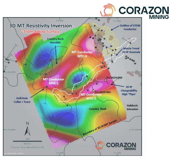
**Figure 6** – MT Resistivity Inversion Image at ~350m below surface. Hot colours depict strong conductivity. "MTC" targets and drill holes **FL2024-060** and **-061** are located on this plan. The location of the MT geophysical survey area within the Lynn Lake Project is shown in Figure 5.
