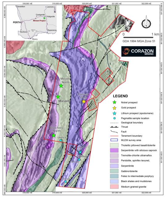
Figure 2 – Miriam Project interpreted geology over aeromagnetic image with sample locations.
